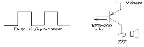
The base current Ib should high enough so that it saturates the collector current of the transistor with the CB load.
